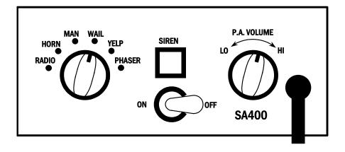
The **OFF/ON** Toggle Power Switch controls the siren power. The siren may be left on any time the vehicle is in operation. The power should be turned off when vehicle is not being used to conserve battery power.
